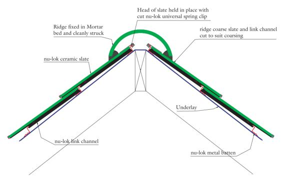
Figure 4: Bedded Ridge Detail
