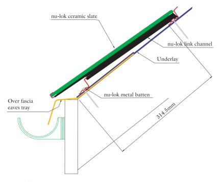
Figure 3: Standard Eaves Detail
