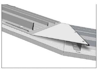
*Fig. 21* Transition flashing combines the attachment techniques of valleys (top of page) with that used with ridge caps (p. 10). Notice the panel set-back that allows proper watershed from the upper panels onto the lower. The less the difference in pitch, as well as the flatter the roof, the greater the amount of set-back, and the more need for a longer lower side on the transition flashing.
