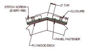
The decking must of course be cut at the ridge to let out hot air. Vent material is either a sponge-like or fibrous material that prevents wind-driven rain, insects, leaves and debris from entering the attic, while at the same time allowing the release of hot air out of the attic. Installation may require caulk to hold the material in place.
