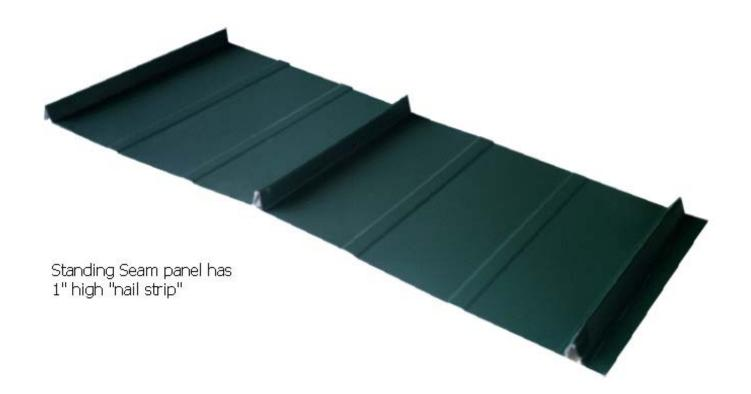
Standing Seam features approximately one-inch high ribs and a net coverage of 16 inches. The "nail strip" and screws that attach each panel are in turn covered by each subsequent panel as each overlapping panel locks into place over the previous one.
