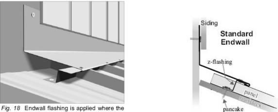
upper slope of a roof meets a wall.
