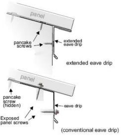
Some installers and do-it-yourselfers elect to install the conventional eave drip (as shown above) along the eave of the building. It is a much easier procedure and simplifies installation and allows for a much faster application of the roofing.
