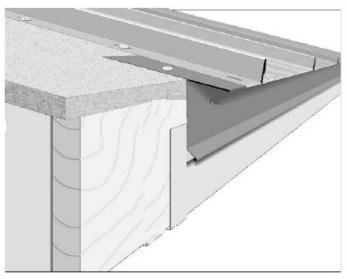
Layered view of eave, showing fascia and extended drip edge, and panel (which is bend on site by installer)
