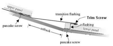
Transition flashing is required when a roof makes a change from a steeper pitch to a lesser pitch. The panels on the upper slope are attached in the same way as valleys. On the lower side, the transition flashing extends over the panels and is attached to Z-flashing with trim screws. Be sure to specify both upper and lower pitches when ordering.
