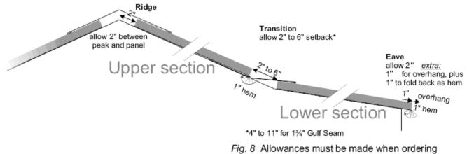
Fig. 8 Allowances must be made when ordering panels to allow for hemming of panels, overhang, ridge venting, and errors.
