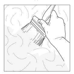
Gently brush on penetrating fluid, or dampen and loosen the coating with steam
