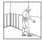
Hold the lower sidewall panel snugly against upper panel.
