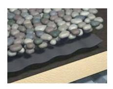
**Ballasted** Ballasted systems are perfect for installations where speed and economy are prime considerations, and the substrate is capable of supporting the system's dead load. Slope must not exceed 2" (50.8 mm). Insulation and membrane are loose-laid with the membrane fastened only at the perimeter. Recommended ballast is smooth, water-worn rocks.
