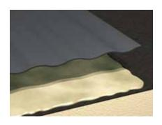
Fully Adhered Fully Adhered systems are ideal for roofs with unusual or oddshaped contours, or where mechanical penetration of the membrane is not desirable. while providing exceptional wind performance and longevity. Once positioned over the substrate, the back of the membrane and the substrate are coated with GenFlex bonding adhesive, allowed to dry, carefully rolled back into position and broomed into place.
