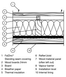
During certain atmospheric conditions metal cools down to the point that condensation forms on the lower side of the sheet, which cannot evaporate through the closed skin of metal. Due to this 'Additional Safety' the two-walled, ventilated roof structure has become the de-facto standard of metal roofings.
