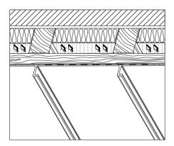
Construction Principle Angle Folding Technique
