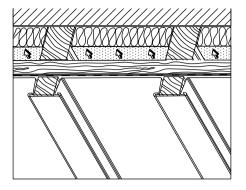
Construction principle of the roll cap technique , for a FalZinc<sup>®</sup> outer wall covering
