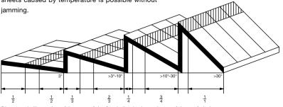
Diagramatic illustration of the area of the fixed clips in dependence of the roof pitch
