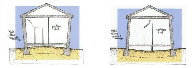
The dome effect causes the walls to tilt outwards and the restraining influence of the roof produces horizontal cracks on the outside wall. These will be wider on the outside surface rather than the inner.
